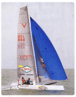
**ABOVE** Mainsheet tension provides a backstay to support the mast when sailing with the spinnaker, with plenty of volume low down in the bows helping to ensure the Viper flies, instead of dives, downwind
